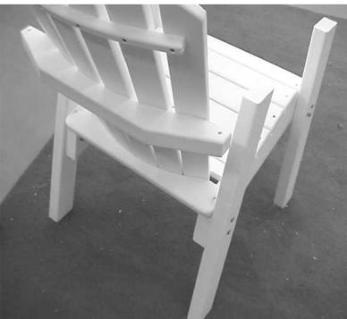
Place chair to standing position. Place Back Assembly on top of mounting surface of Rear Legs. Push Back Assembly forward until it is aligned with Seat Assembly (Left Picture). Hold Back Assembly in place and install using (2) 1-3/4" Phillip's Head Screw into pre-drilled holes on both sides of Assembly (Right Picture)
