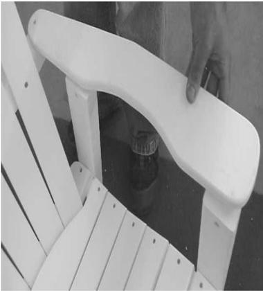
Place Arm Assembly on top of Front Leg and Upper Back Yoke (Left Picture). Align hole in Arm Assembly with the hole located at the top of the Front Leg. Install using (1) 2-3/4" connector bolt through hole in underarm support and through Front Leg with flat & lock washers and nuts (Right Picture). Do not tighten at this time. Repeat process on other side.
