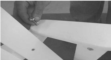
Install (1) 2-3/4" connector bolt through pre-drilled hole through arm and through upper back yoke (Left Picture). Finger tighten flat & lock washers and nuts. Do not tighten at this time. Repeat process for opposite side.
